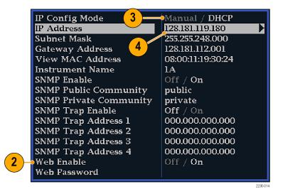
6. Start your Web browser and type the network address of the instrument (from step 4) into the URL entry box like this: 1 http://123.123.123.
