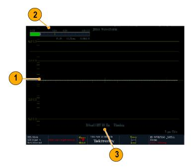
**High-Pass Filter.** The high-pass filter bandwidth setting allows you to show only jitter terms above the selected filter frequency. When you select a filter setting, depending on the active input signal, you select the jitter measurement type (Timing, Alignment, or neither, as defined by the SMPTE standard). Use the High Pass Filter soft key to select the lowest settings to measure timing jitter and the higher settings to measure alignment jitter.
