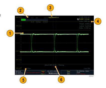
At the end of a long cable, the eye diagram may appear so noisy that there is little or no discernable opening. In this situation, limited use of the eye diagram is still possible by selecting Equalized Eye mode. The equalizer compensates for the effects of cable length by applying an inverse response function and then reslicing the signal to a logic level. This causes amplitude information to be lost, but preserves the effects of jitter in the signal.
